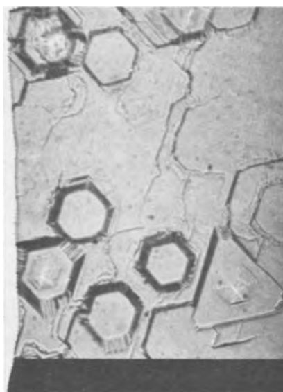
Fig. 7. An example of macrosteps on side faces of truncated pyramids. 5 \text{ ma/cm}^2 in the presence of n -decylamine (600X).
