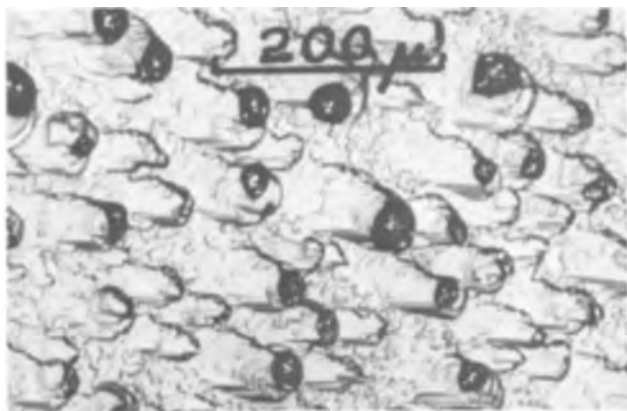
Fig. 1. Silicon-aluminum alloy globules and associated etch pits on a (\bar{1}\bar{1}02) alumina surface.
