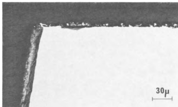
Fig. 11. Section perpendicular to specimen showing Potter and Mann growth on vertical face, Bloom growth on horizontal face. The specimen was oxidized in 15% NaOH in a nonconditioned pressure vessel for 63¼ hr to give a Bloom film on all faces; the Bloom film was removed from the vertical face and the specimen re-oxidized for 70¼ hr in the same pressure vessel.
