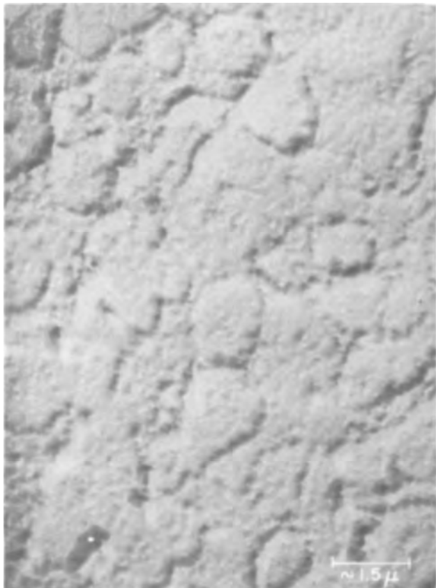
Fig. 4. Chemical oxide, electron micrograph, replica. Magnification ca. 23,330X.
