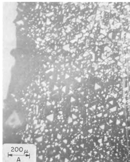
Fig. 4. Growth at 1700°C on etched, natural (0001) SiC surface when mole ratio was 0.3%.
