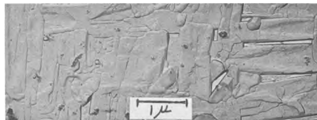
Fig. 10. Alloy layer on the {100} face of iron formed by slowly heating the single crystal for 60 sec.
