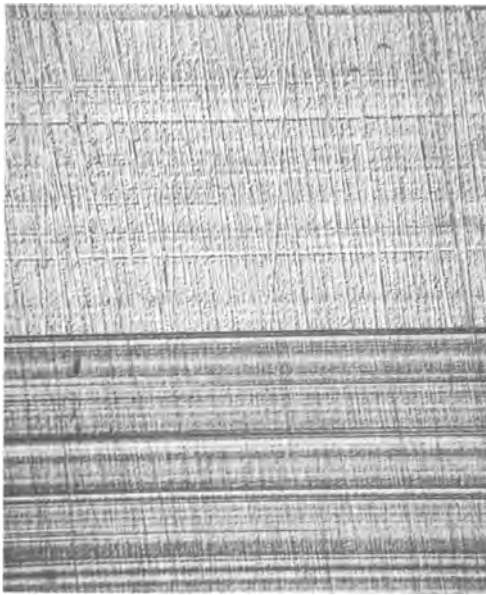
Fig. 1. Impurity striations on a rotational twin; the upper part is a (211) and the lower part a (\bar{2}\bar{1}\bar{1}) plane. The latter one is employed throughout this study for revealing the various types of striations. Magnification 95X.
