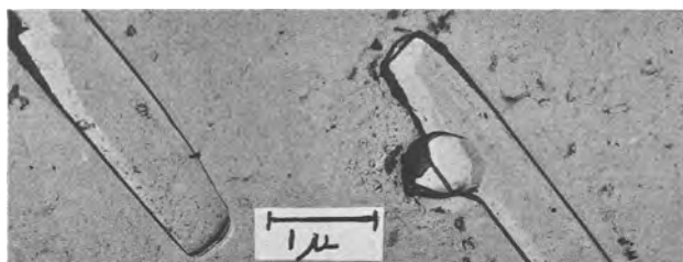
Fig. 11. Alloy layer on electropolished {100} face of iron
