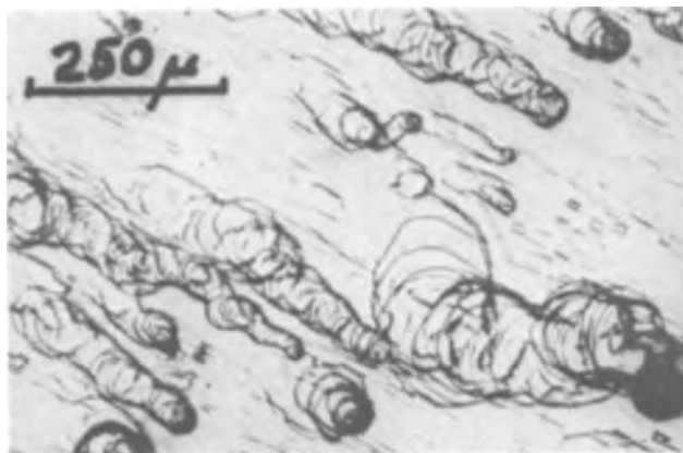
Fig. 2. Tracks left on the (\bar{1}\bar{1}02) alumina surface by migrating alloy droplets.
