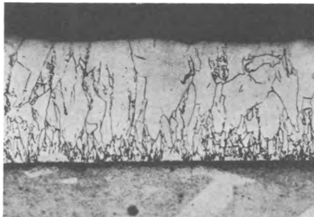
Fig. 3. Cross section of zirconium diboride coating (X150)
