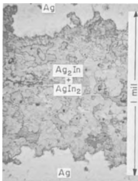
Fig. 8. Ag-In SLID bond made at 200°C for 30 min. Etchant: 2g K 2 Cr 2 O 7 , 8 ml H 2 SO 4 ; 4 ml NaCl (sat. sol.), 400 ml H 2 O; swab for 10 to 30 sec; at temperatures as low as 200°C transformation of indium to higher melting phases is complete.
