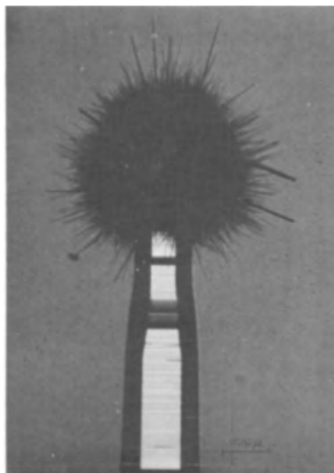
Fig. 4. Uncontrolled VLS growth resulting from nucleation of silicon crystals in liquid alloy. Magnification 250X.
