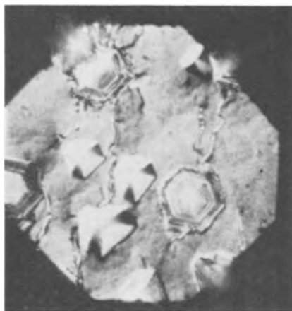
Fig. 2. Electrodeposit at an average thickness of deposit corresponding to 10 coulomb/cm 2 showing hexagonally shaped and triangular pyramids. Current density i = 5 \text{ ma/cm}^2 (600X).
