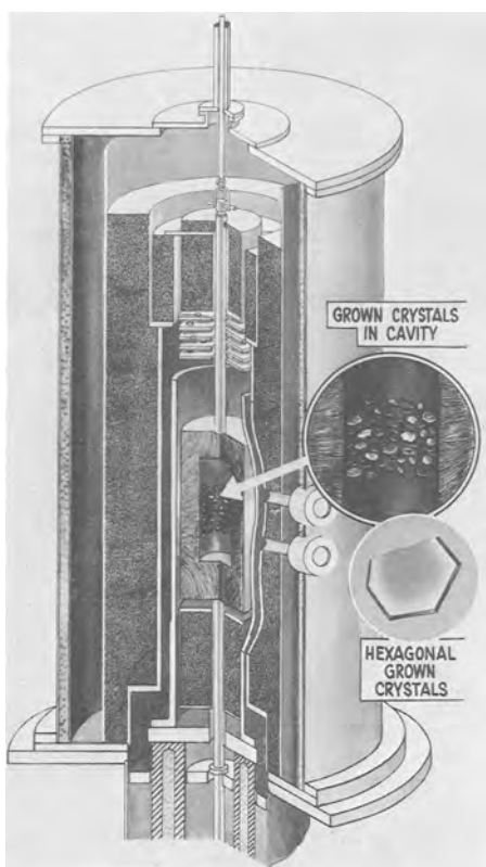
Fig. 1. Schematic drawing of 2600°C silicon carbide crystal growth furnace showing water-cooled envelope, powdered graphite insulation, and crucible with crystals attached to cavity wall.
