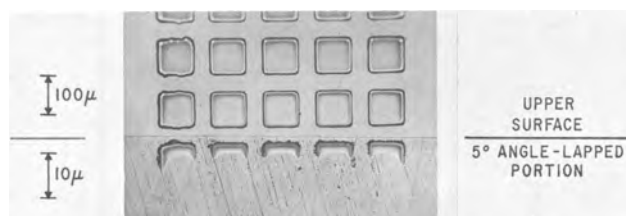
Fig. 1. Micrograph showing 5° angle-lapped section through holes etched into GaAs with an unstirred bromine-methanol (1:1000) solution.
