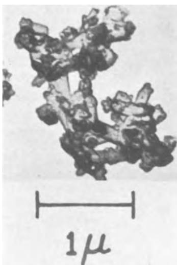
Fig. 2b. A cluster of small prismatic crystals
