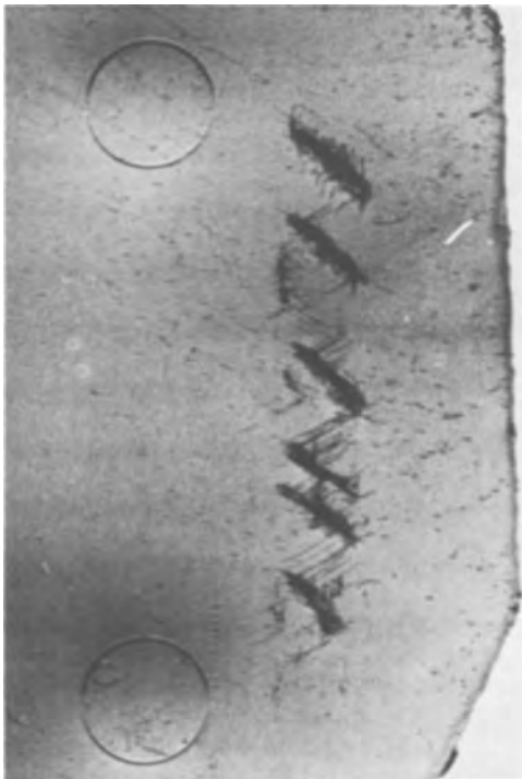
Fig. 4. Small area topograph of diffused silicon wafer illustrating dislocations nucleating at scratches on the wafer surface.
