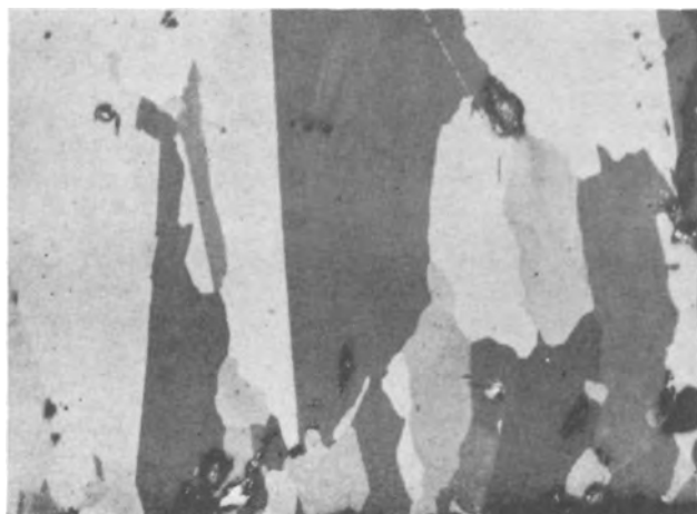
Fig. 2. Piece of detached Zr plate (X150)*
