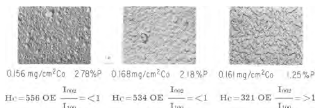
Fig. 4. Electron micrographs for cobalt-phosphorus films with increasing phosphorus concentration at constant cobalt weight. Magnification 10,000X.
