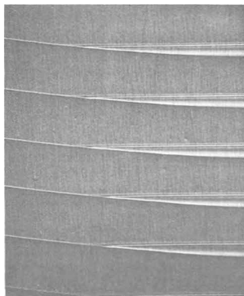
Fig. 10. Rotational striations in the on core-off core transition region. The absence of nonrotational striations is due to the low impurity concentration (6 mg Te in 50g melt). Magnification 95X.
