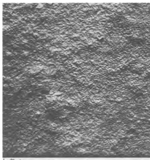
Fig. 12. Electronmicrograph of a highly oriented crystalline CdS film.
