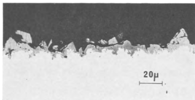
Fig. 2. Normal section of \text{Fe}_3\text{O}_4 growth on the inner surface of a mild steel capsule. Oxidized for 72¼ hr in 15% NaOH.
