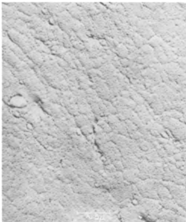
Fig. 6. Oxide formed with \text{NH}_4\text{OH} , electron micrograph. Magnification ca. 6700X.
