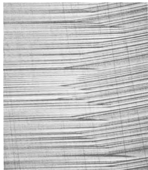
Fig. 4. Nonrotational impurity striations in a heavily doped crystal (60 mg Te in 50g melt). The striations are straight in the "on core" region on the left and exhibit curvature in the "off core" region on the right hand side of the photograph. The on core-off core interface is corrugated in appearance. Compare with striations No. 1 in Fig. 3. Magnification 95X.
