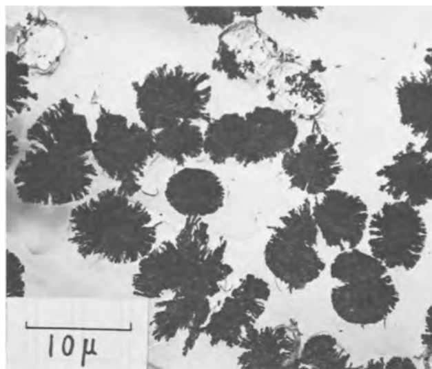
Fig. 3. Spherulite-like crystals of \alpha -cristobalite found on the quartz boat after downward solidification of GaAs.
