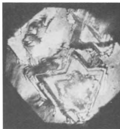
Fig. 8. An example of possible twinning (600X).
