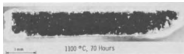
Fig. 6. Cross section of GaP plate oxidized in oxygen. Some sample as 1100°C, 70 hr in Fig. 6.
