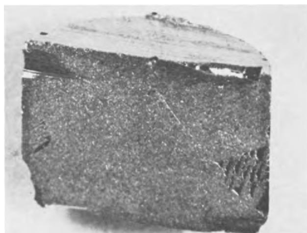
Fig. 3. Vertical cross section of the top end of a PbTe ingot obtained by this method.
