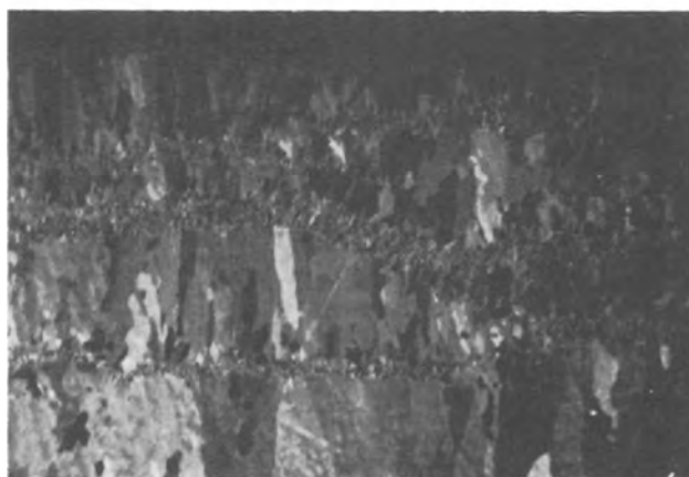
Fig. 6. Zirconium-titanium alloy (X150)
