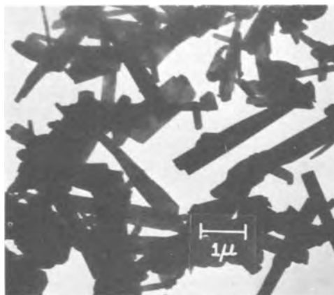
Fig. 1a. Electron micrograph of \text{PbO} \cdot \text{PbSO}_4 crystals. These appear to be rather thin blunted needles and were the smallest in average size of the basic sulfates prepared for this study.
