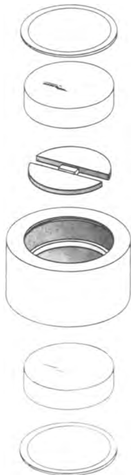
Fig. 1. Exploded view of the cell without the thermostating clamp
