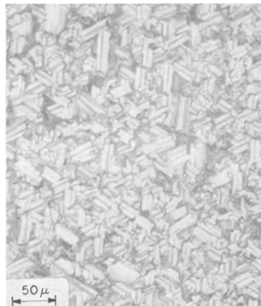
Fig. 3. Growth at 1650°C on natural (0001) SiC surface
