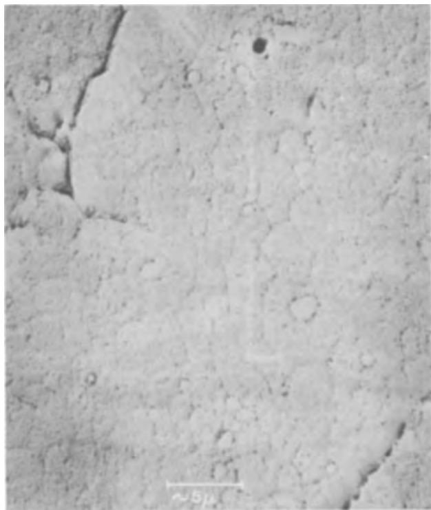
Fig. 8. Oxide formed with H_2O , electron micrograph. Magnification ca. 6700X.
