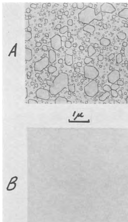
Fig. 6. Oxide formation on annealed (110) faces of copper; a, 5 min in 0.05N CuSO 4 at 30.0°C, initial pH 4.3; b, 5 min immersion in 0.05N Cu(OAc) 2 at 30°C, pH 4.3. Magnification 15000X before reduction for publication.
