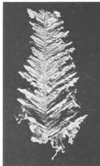
Fig. 5. Typical silver dendrite grown from 3% AgCl solution in LiCl-KCl at 450°C. Current density, 2.28 ma/cm 2 ; overpotential, 5.3 mv.
