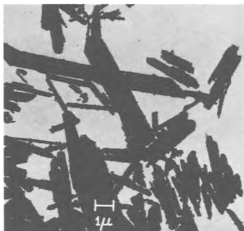
Fig. 1b. Electron micrograph of 3\text{PbO} \cdot \text{PbSO}_4 \cdot \text{H}_2\text{O} crystals. The wide variation in size of these slender needles is apparent in this photograph. The surfaces of these crystals are covered with protrusions which may be incipient or vestigial dendritic arms.
