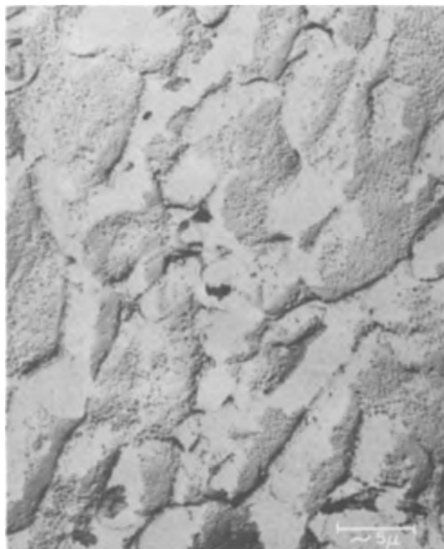
Fig. 7. Oxide formed with \text{H}_2\text{O}_2 , electron micrograph. Magnification ca. 6700X.
