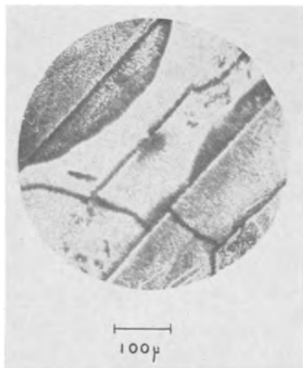
Fig. 2. Cracks in germanium grown on silicon from a tin solution after 30-sec white etch.
